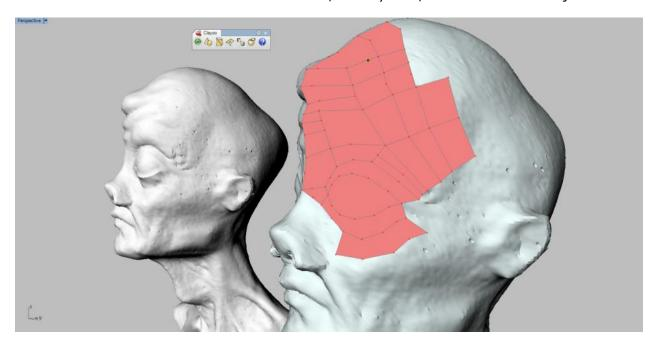
When you run the command you have to select a mesh and then pick vertex by vertex to create the surface faces on the selected mesh. With Shift we can drag the vertex.
